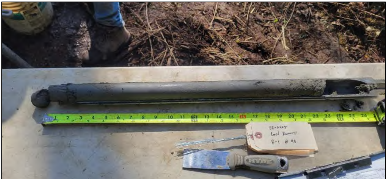
Image 5. View of sample taken at 40 feet BGS from boring B-1 exhibiting Middle Glaciomarine Drift deposits.
